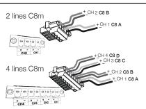
Euroblock 4/8-p amplifier output wiring
