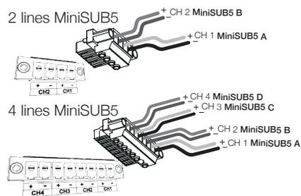
Euroblock 4/8-p amplifier output wiring
