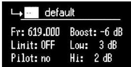
The configuration saved before the loading of the clone is saved on the clone named “default”, therefore loading the default “clone” allows to return with the previous settings. The following arrows displayed near the clone number indicates the currently clone loaded.
