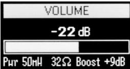
*NOTE: When the volume knob is rotated, appears a screen with a volume bar and the values of Pwr limit, Output load and Vol. boost*
