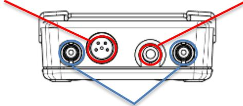
SMA connectors Antenna A & B
