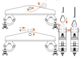
Alternatively, connect the TRUSS BRACKET 30/40HC to the lifting hook. Open the hook, place the pin (a) of the TRUSS BRACKET 30/40HC in it and secure the hook again.
