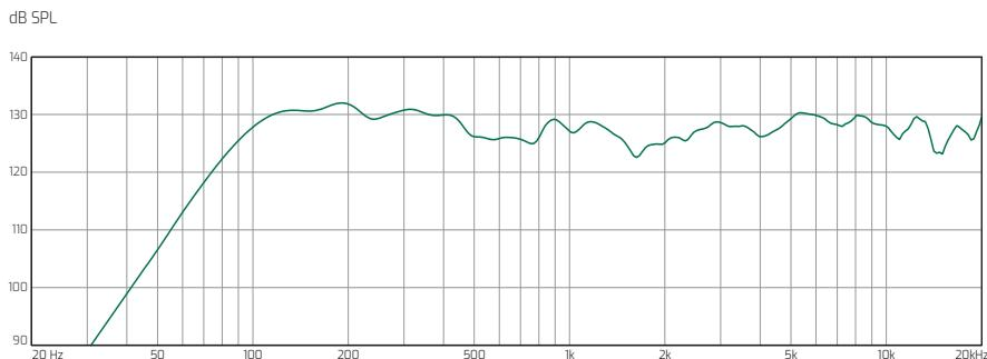
The graph shows the frequency response for a 1-watt swept sine signal in an anechoic environment ( $4\pi$ ), measured at 3 m and scaled down at 1 m.
