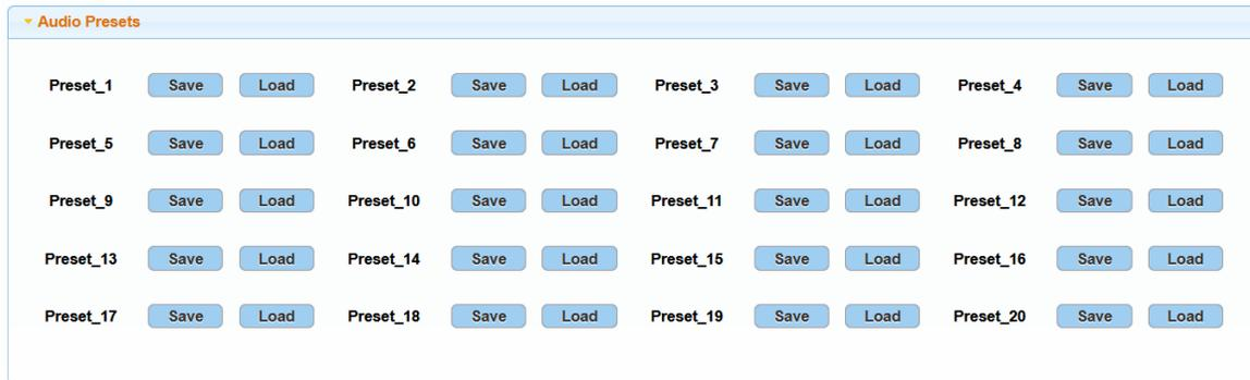
This section saves/loads the audio input/output switch settings to or from the Matrix.
