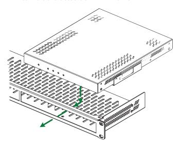
3. Attach the NHD-124-TX encoder(s) to the NHD-124-RACK-1U main shelf using the supplied screws.
