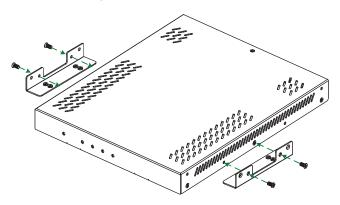
Position the NHD-124-TX encoder(s) through the NHD-124-RACK-1U front face cutout(s) so that the front or rear face of the encoder(s) is flush with the front face of the NHD-124-RACK-1U.
