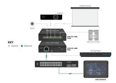
The SYN-CTL-HUB controller can work with the SYN-TOUCH10 touchpad (or any third-party controllers) to control the attached peripherals (e.g. TVs, curtains) through RS-232, IR and/or relay commands.
